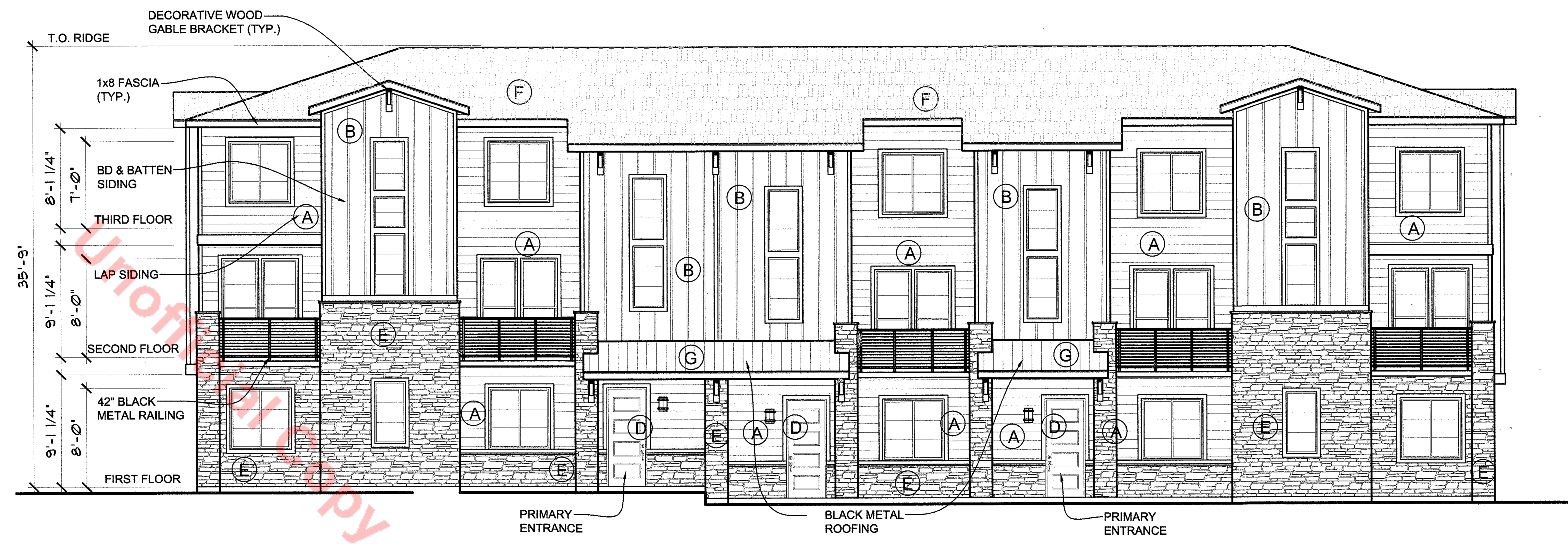
FRONT ELEVATION - 5 UNIT BUILDING
