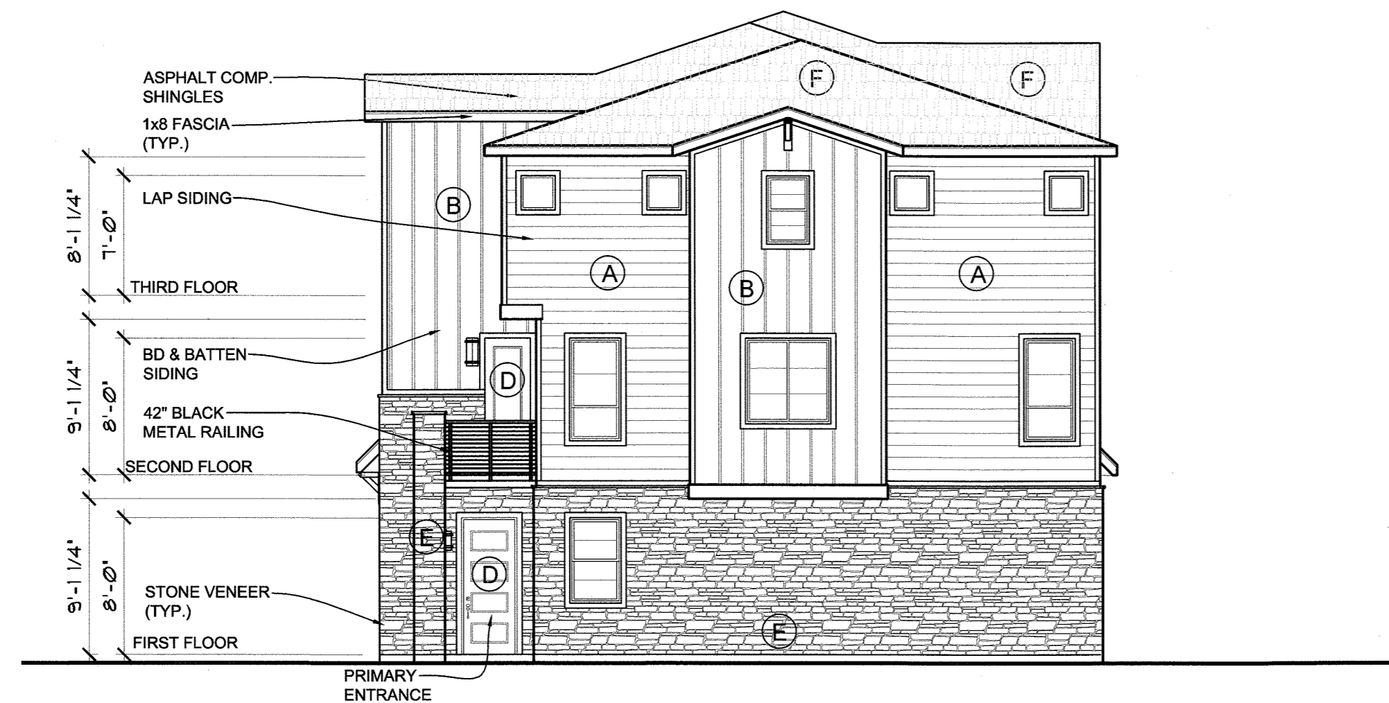
RIGHT ELEVATION - 4 UNIT BUILDING
