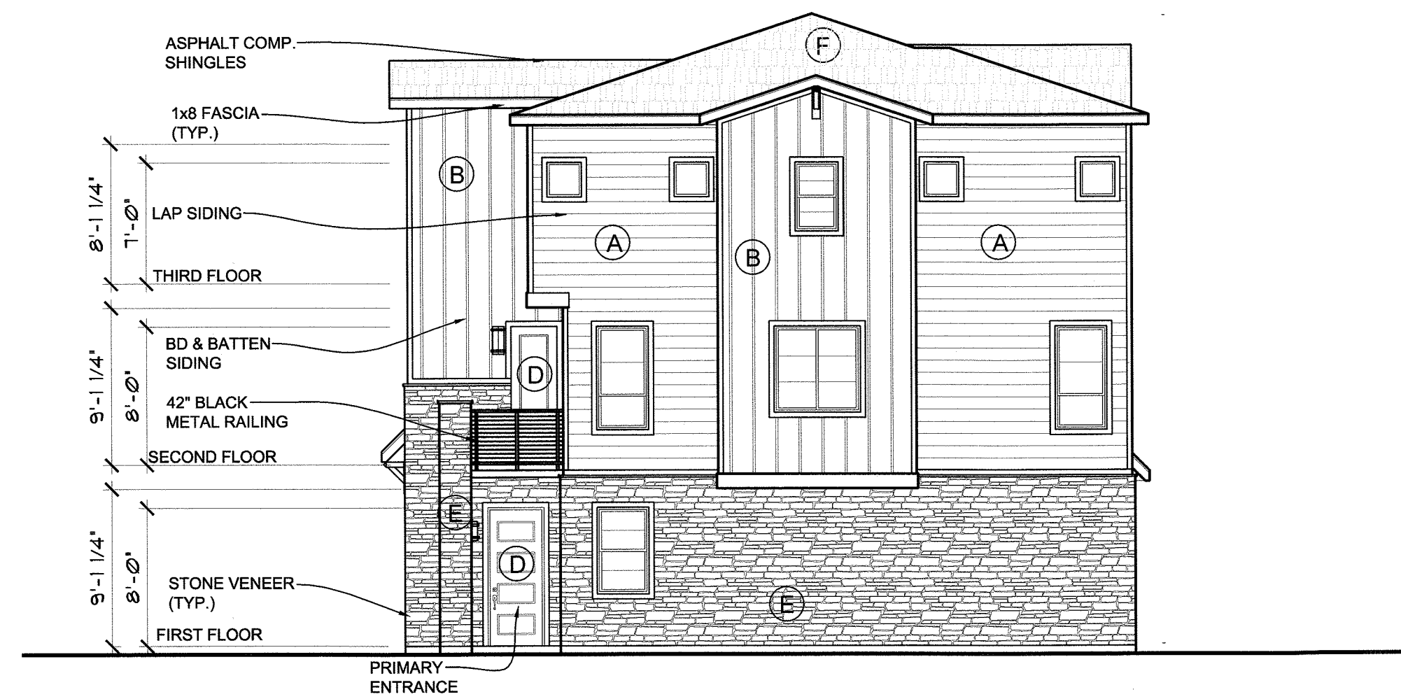
RIGHT ELEVATION - 5 UNIT BUILDING
