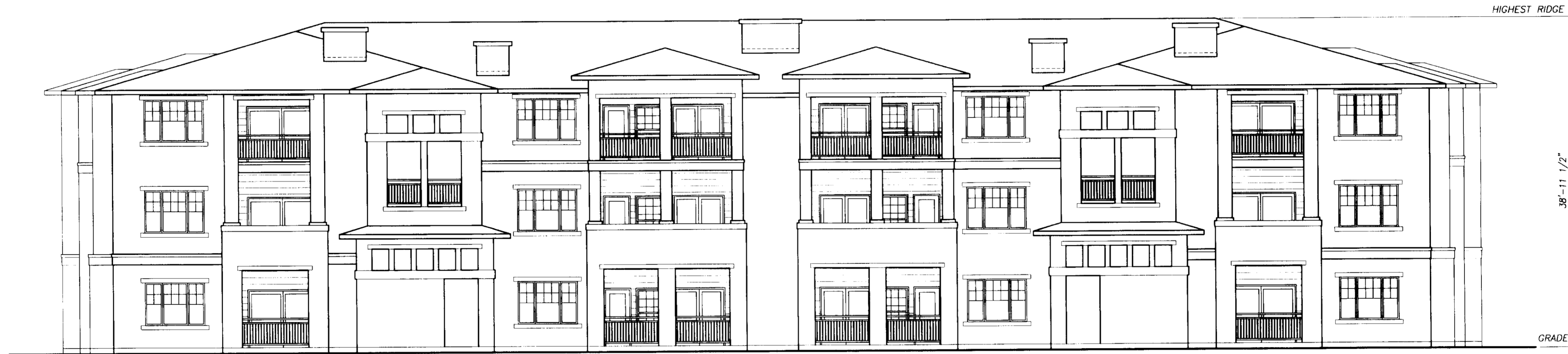
2 REAR EXTERIOR ELEVATION BLDG. TYPE VII-3 SCALE : 1/8" = 1'-0"
