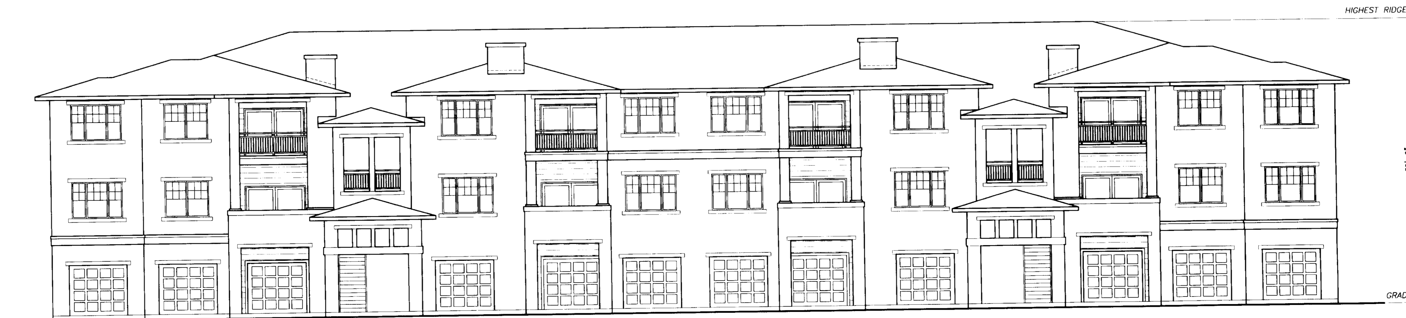
1 FRONT EXTERIOR ELEVATION BLDG. TYPE VIII-3T SCALE: 1/8" = 1'-0"
