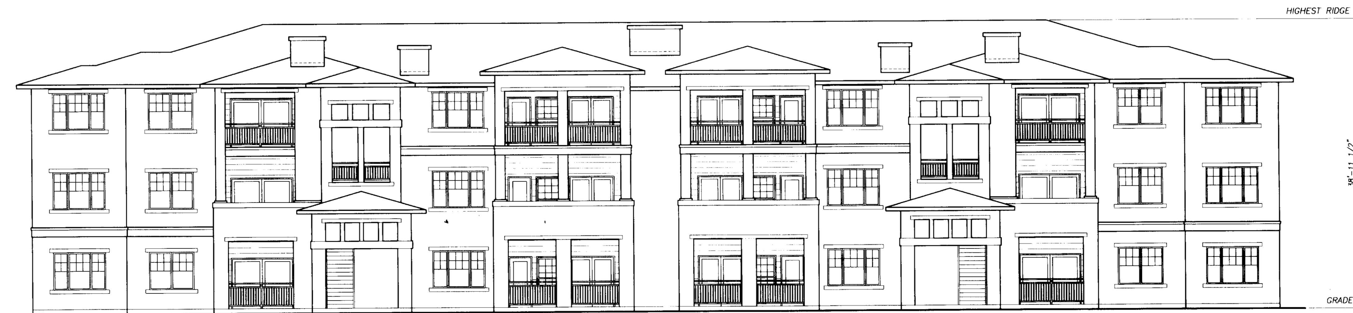
1 FRONT EXTERIOR ELEVATION BLDG. TYPE VII-3 SCALE : 1/8" = 1'-0"
