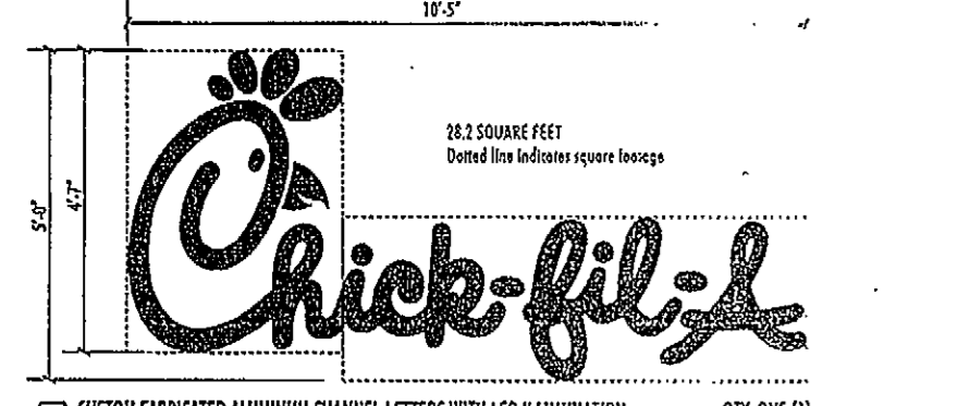
B CUSTOM FABRICATED ALUMINUM CHANNEL LETTERS WITH LED ILLUMINATION Scale: 1/2" = 1'-0" QTY: ONE (1) AREA: 28.2 SQ. FT.
