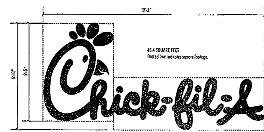
A CUSTOM FABRICATED ALUMINUM CHANNEL LETTERS WITH LED ILLUMINATION Scale: 1/2" = 1'-0" QTY: THREE (3) AREA: 45.4 SQ. FT.
