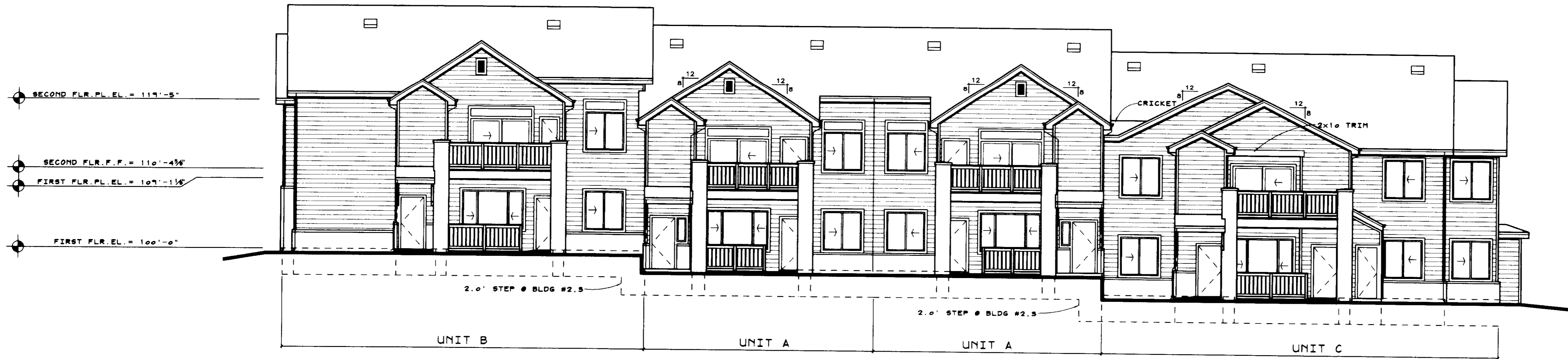
BUILDING TYPE III FRONT ELEVATION REAR ELEVATION TO BE MIRRORED NOTES TO BE SIMILAR TO NOTES BELOW 1/8" = 1'-0"
