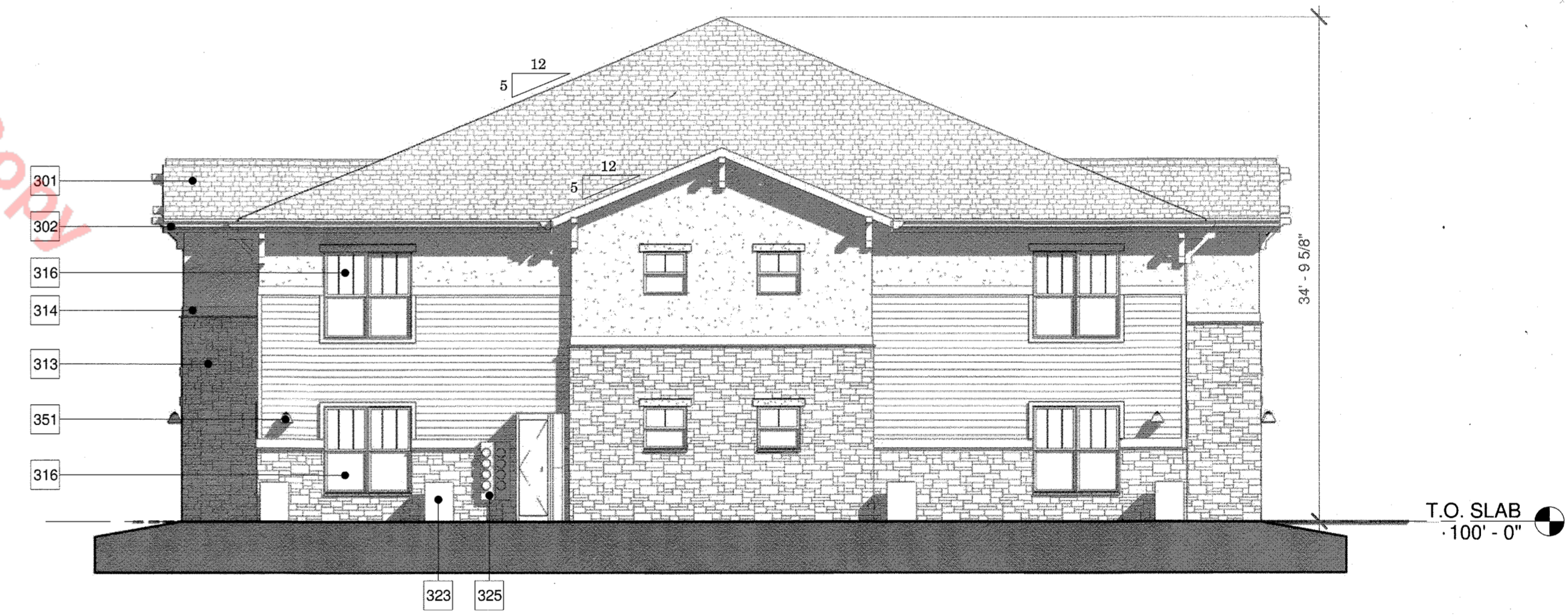
BUILDING 4 & 5 EAST ELEVATION 1/8" = 1'-0"
