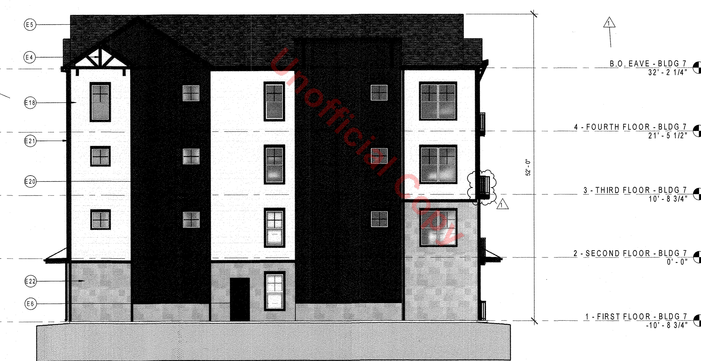
2 RIGHT ELEVATION BUILDING 7 1/8" = 1'-0"
