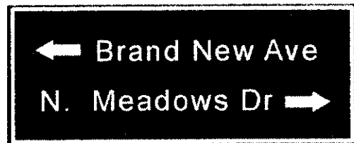
Post on US 85 SB off-ramp (Reverse arrows for NB off-ramp)
