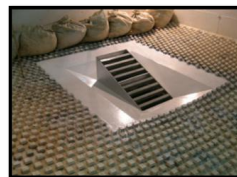
CDOT Type D Inlet in Corrieo (20° Incline & Depressed)
