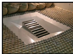
CDOT Type D Inlet in Corrieo (10° Incline & Depressed)
