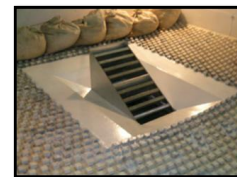
CDOT Type D Inlet in Corrieo (30° Incline & Depressed)
