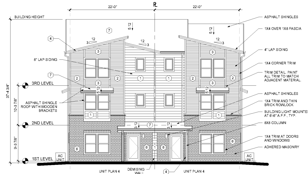
1 DUPLEX - FRONT ELEVATION - MID-CENTURY MODERN 1/8" = 1'-0"
