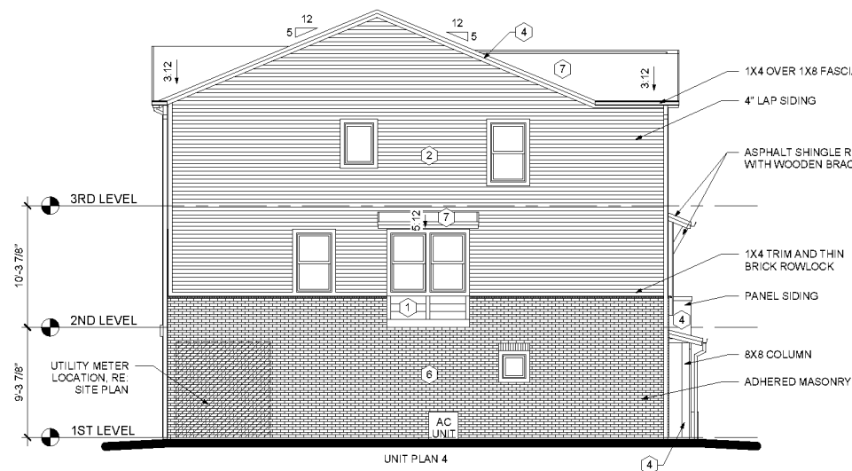
3 3-PLEX - LEFT ELEVATION - MID-CENTURY MODERN 1/8" = 1'-0"
