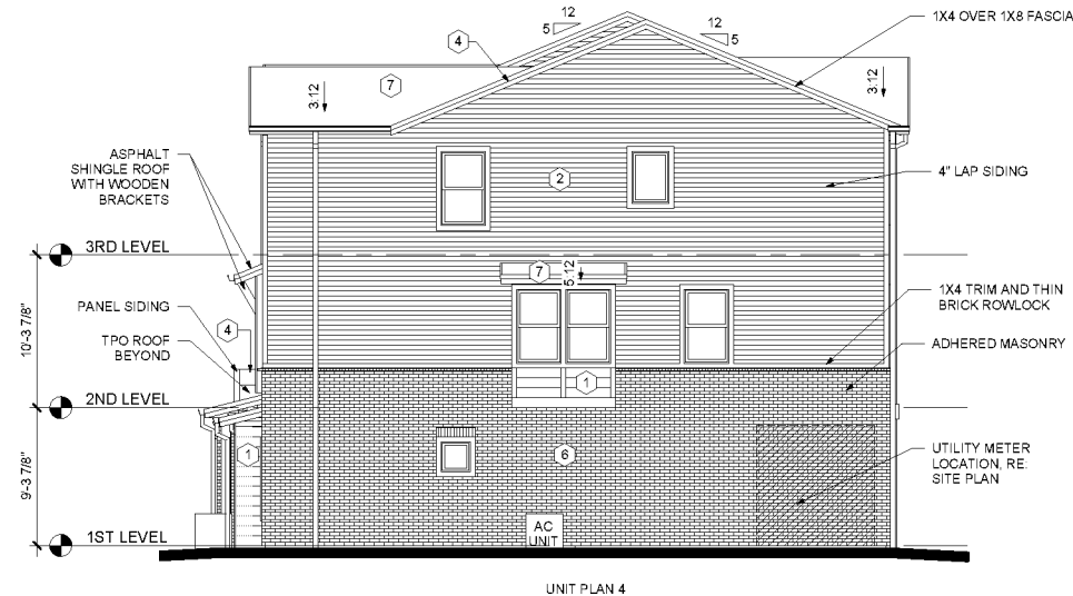
2 4-PLEX - RIGHT ELEVATION - MID-CENTURY MODERN 1/8" = 1'-0"
