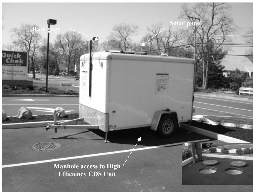
Figure 7 View of Mobile Monitoring Unit (MMU) installed at the Manasquan Savings Bank study site
