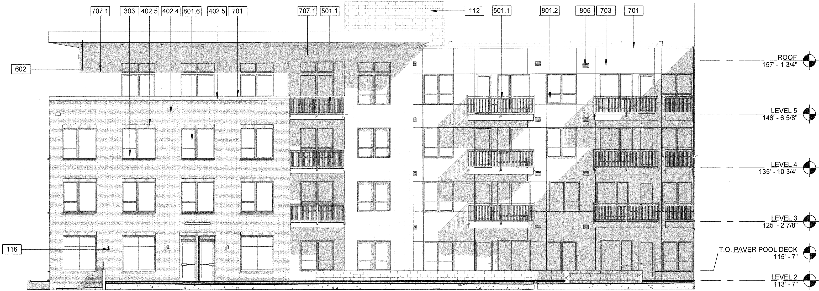
2 BUILDING 5 - POOL DECK NORTH ELEVATION 1" = 10'-0"
