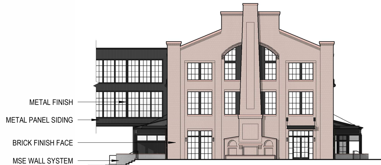
BUILDING 1 - WEST ELEVATION
