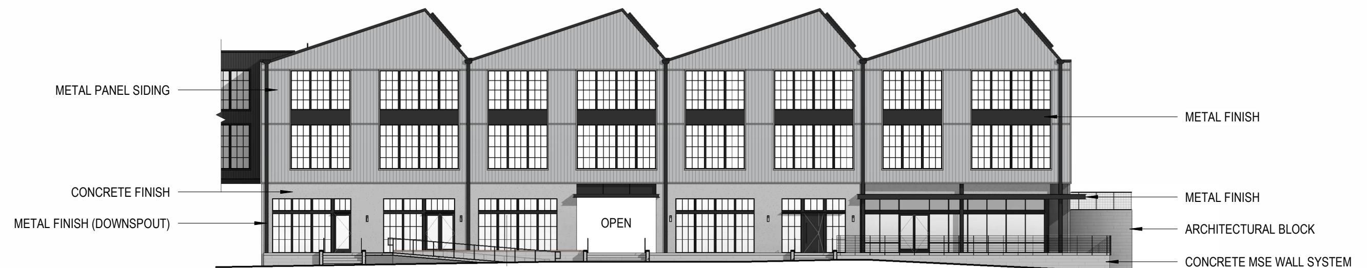
BUILDING 1 - EAST ELEVATION
