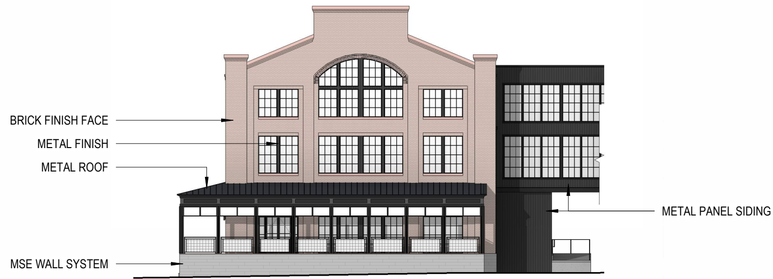
BUILDING 1 - EAST ELEVATION
