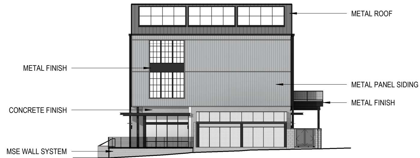
BUILDING 1 - NORTH ELEVATION
