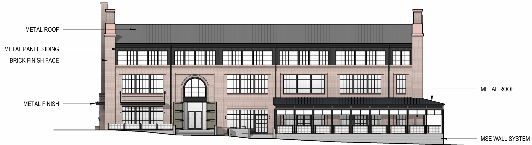
BUILDING 1 - SOUTH ELEVATION
