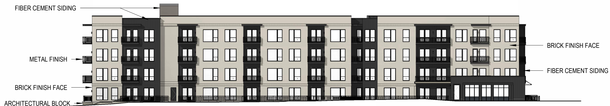
BUILDING 4 - WEST ELEVATION
