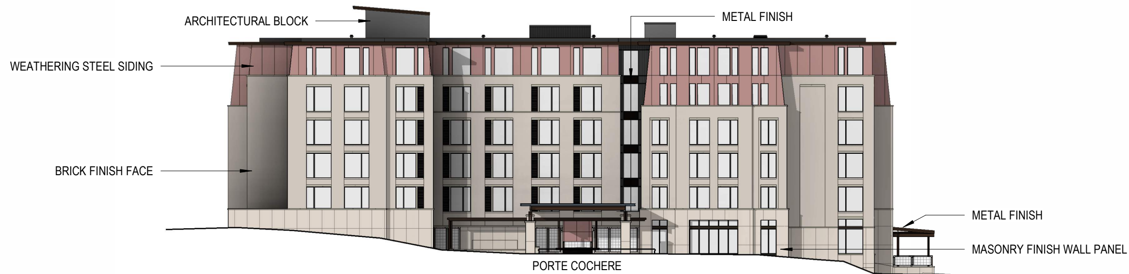
BUILDING 2 - WEST ELEVATION
