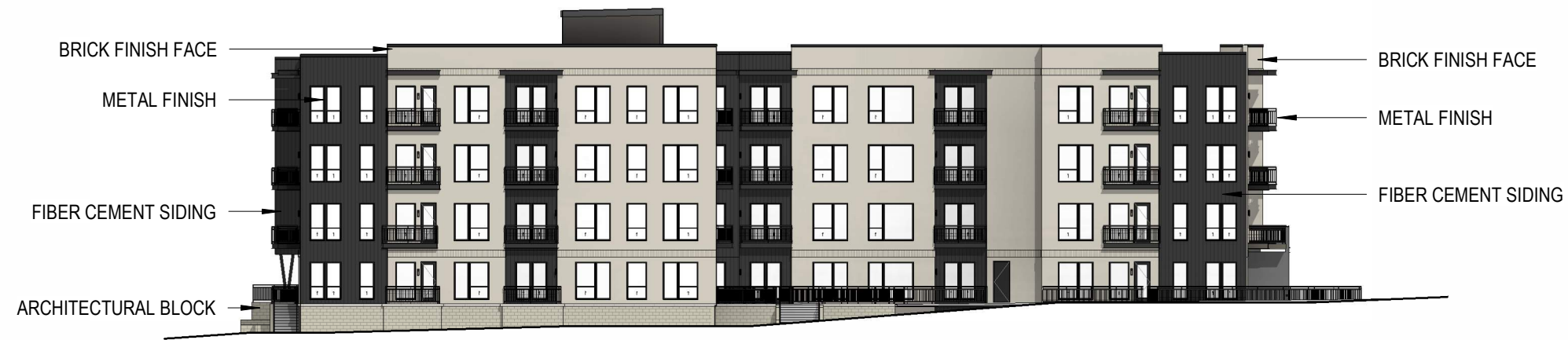
BUILDING 4 - NORTH ELEVATION
