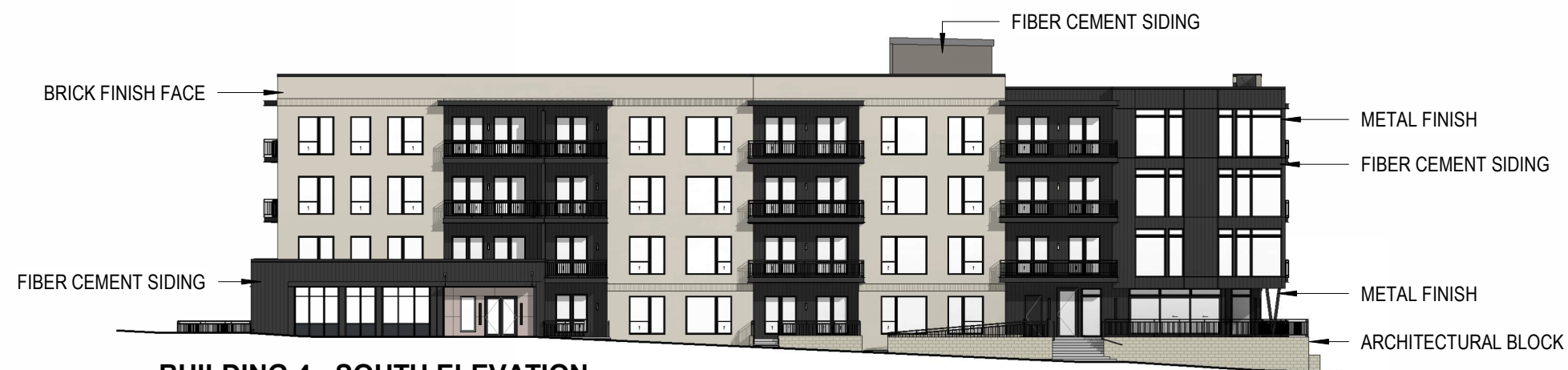
BUILDING 4 - SOUTH ELEVATION
