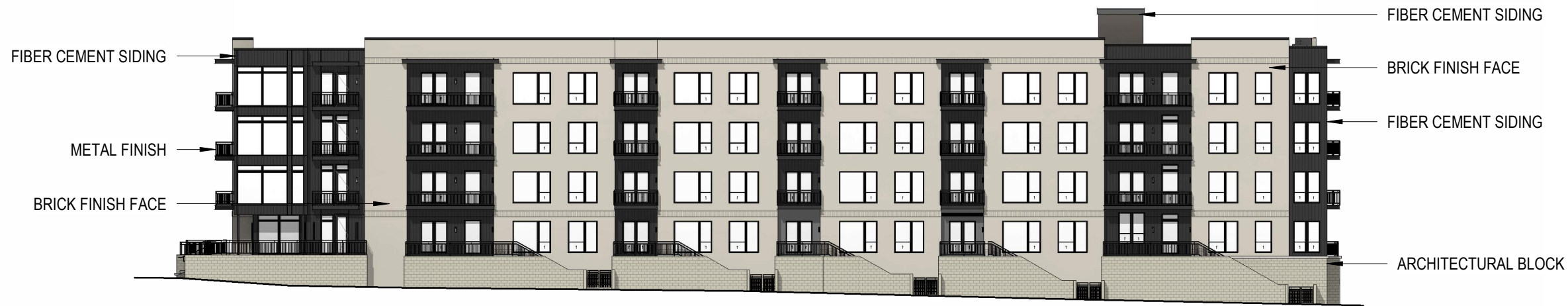
BUILDING 4 - EAST ELEVATION
