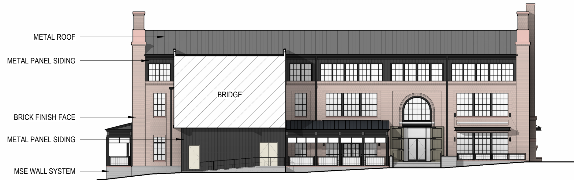
BUILDING 1 - NORTH ELEVATION
