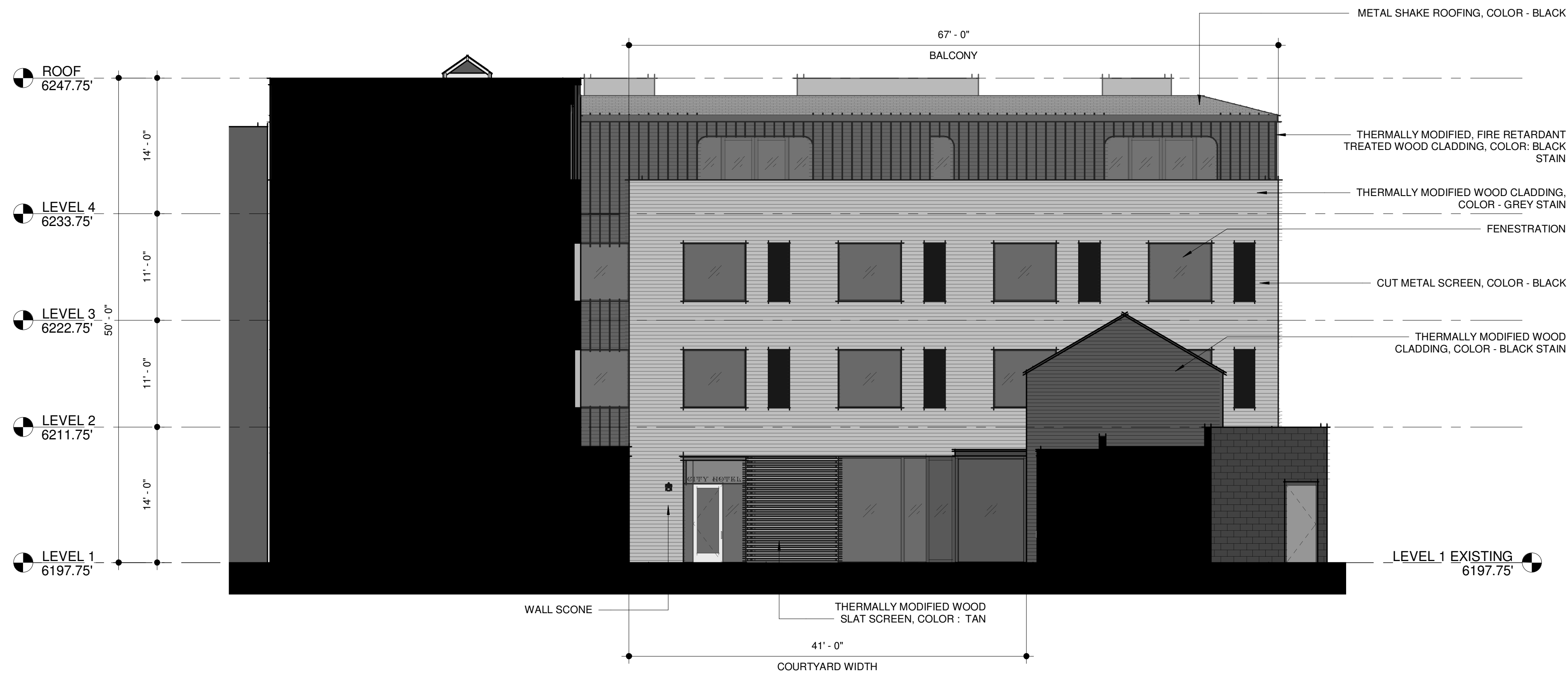
② ELEVATION WEST COURTYARD - SDP 1/8" = 1'-0"
