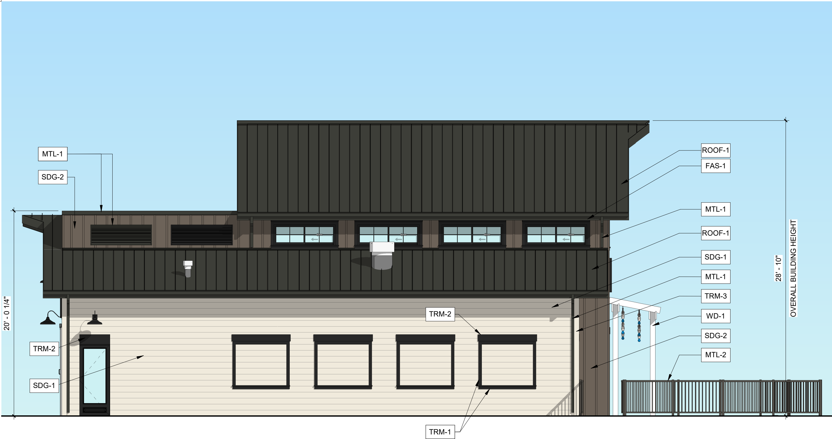
4 BUILDING ELEVATION - NORTH 3/16" = 1'-0"
