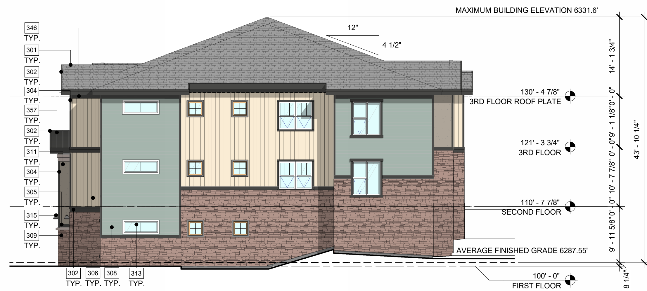
4 BUILDING 1 NORTH ELEVATION 1" = 10'-0"
