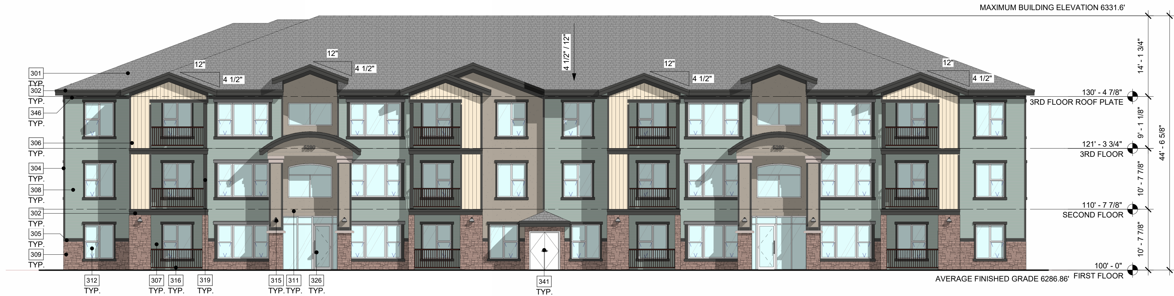
1 BUILDING 1 EAST ELEVATION 1" = 10'-0"
