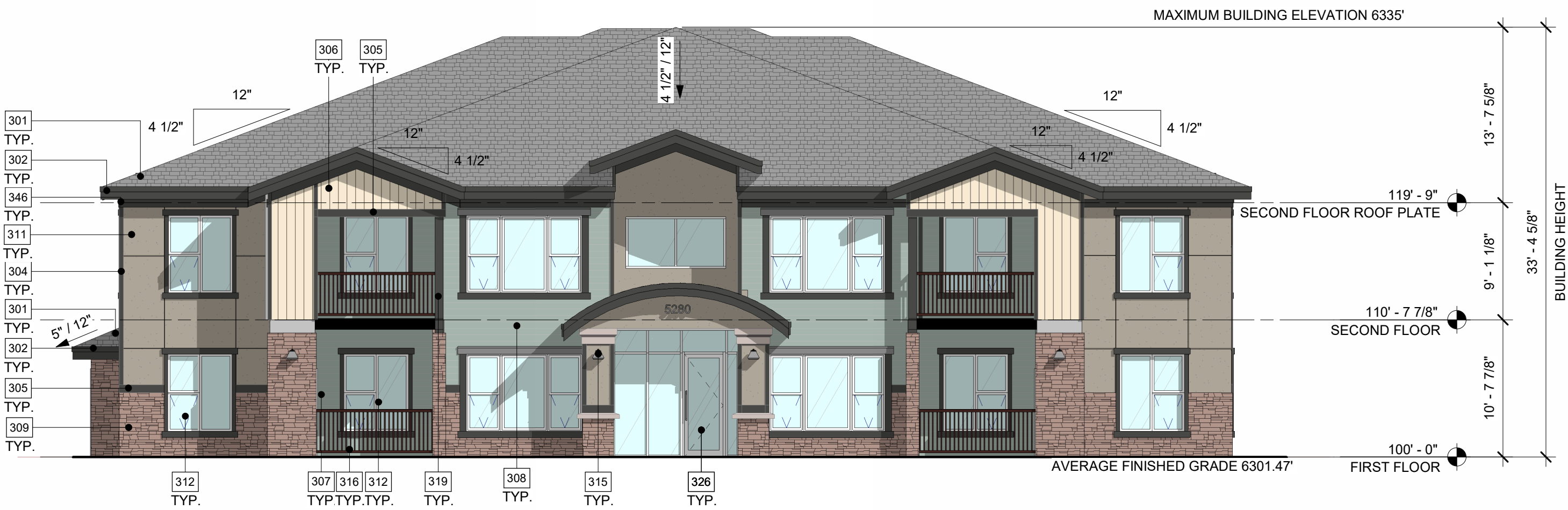
1 BUILDING 5 EAST ELEVATION 1/8" = 1'-0"
