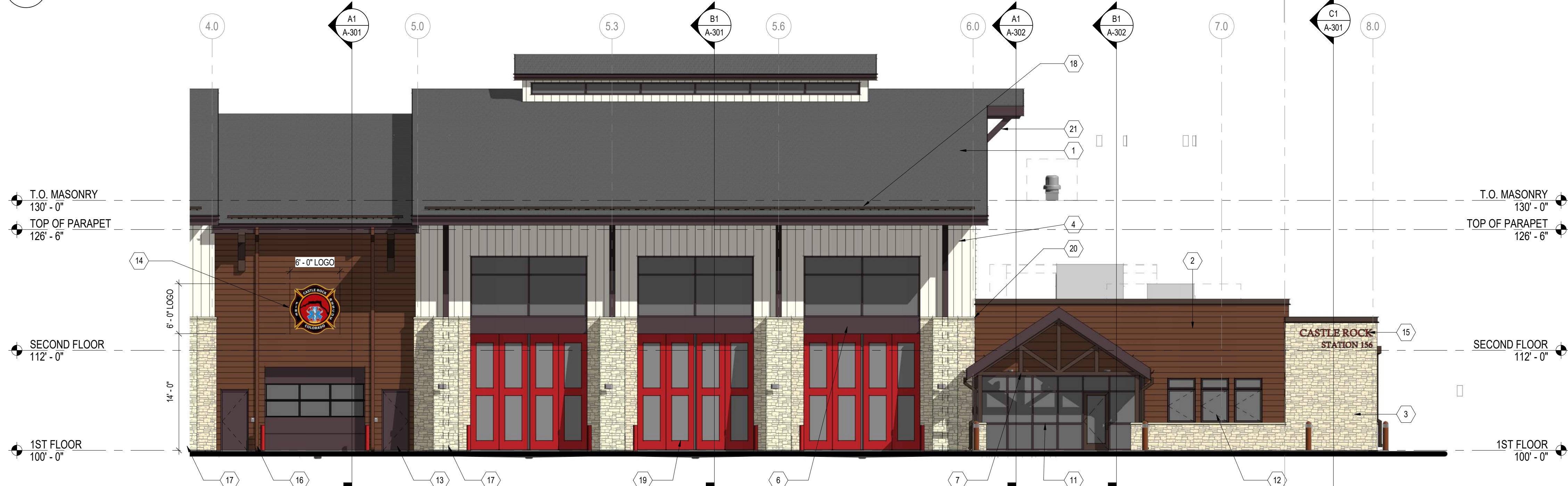
WEST (FRONT) ELEVATION - FIRE STATION SIDE
