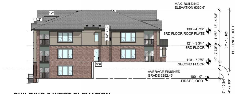
3 BUILDING 3 WEST ELEVATION 1/16" = 1'-0"
