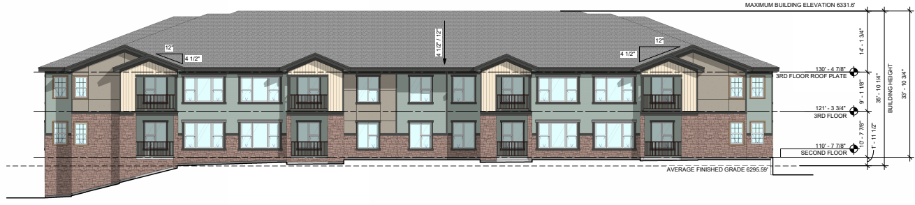
3 BUILDING 1 WEST ELEVATION 1" = 10'-0"
