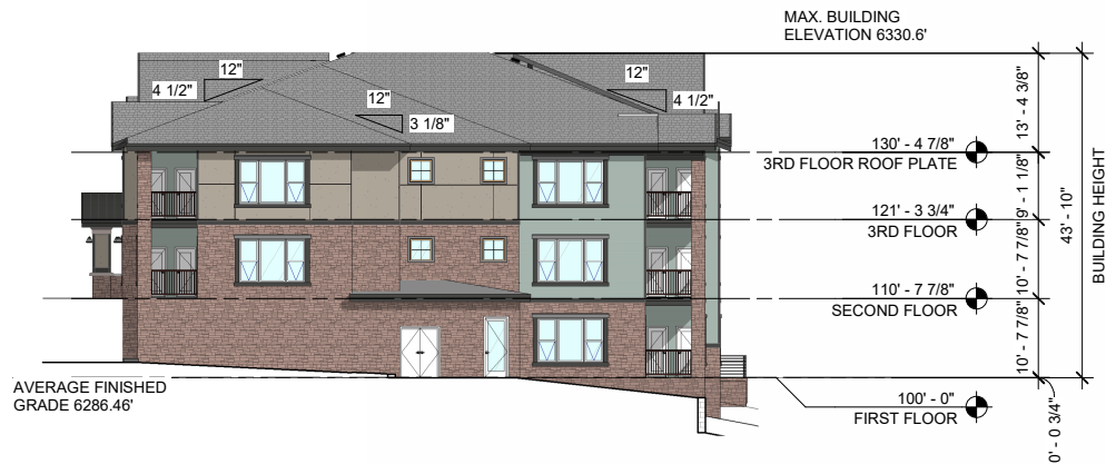
4 BUILDING 3 EAST ELEVATION 1/16" = 1'-0"
