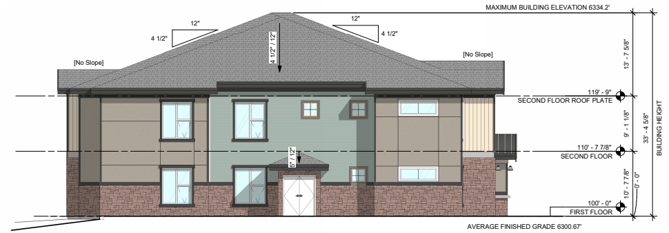
2 BUILDING 4 WEST ELEVATION 1/8" = 1'-0"
