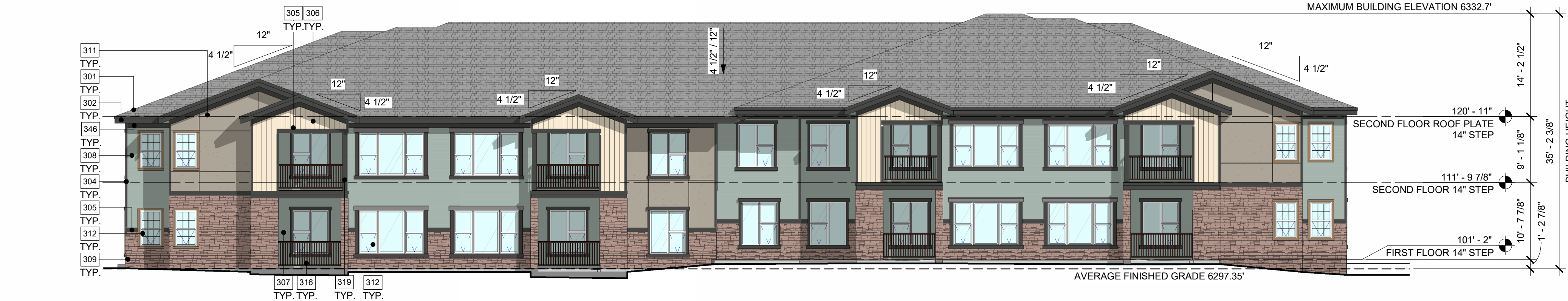
3 BUILDING 2 NORTH ELEVATION 1" = 10'-0"
