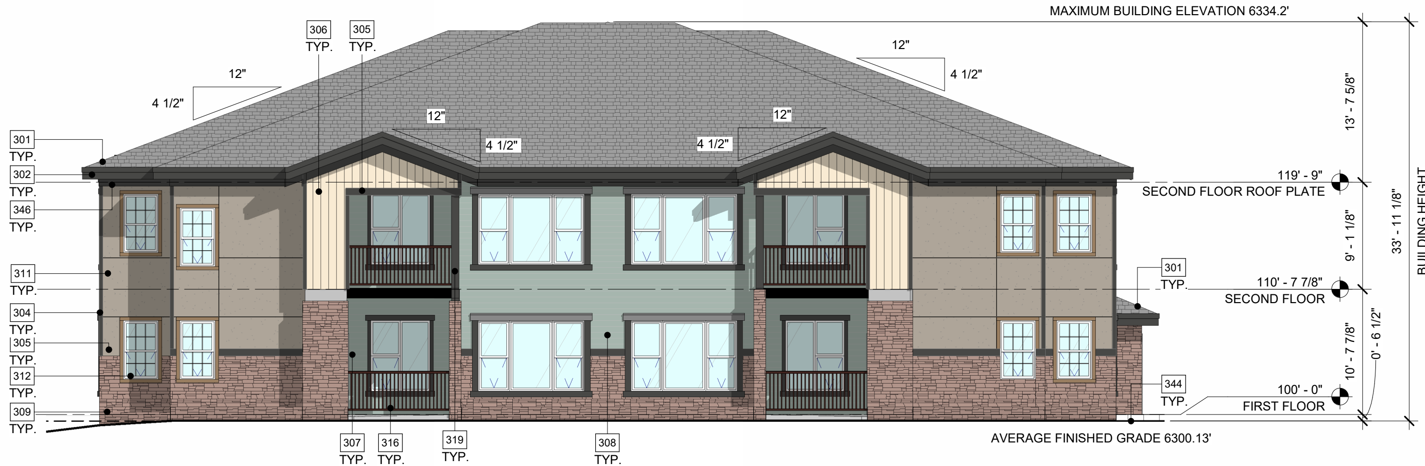
3 BUILDING 4 NORTH ELEVATION 1/8" = 1'-0"
